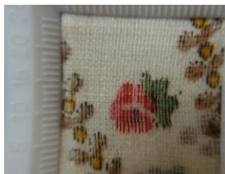
Detail of printed fabric with silk warps (running horizontally in this image) and wool wefts
